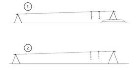
KOMPAN cableways are available for flat or natural sloped surroundings and for surface or in-ground installation. Further the cableways can be supplied with one or two cables for children to ride together in friendly competition. For flat surroundings a starting mound or platform is needed to use the cableway.
