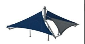
Sails of commercial 95 high density PE knitted specially for sun-shade structures. The sails are treated with UV stabilizers to ensure a long lifetime. The sails are supported by a hot dip galvanized steel frame and tightened by stainless steel devices.
