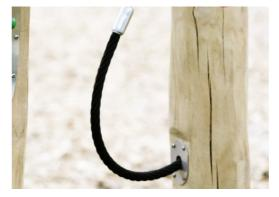
Ropes are made of UV-stabilised PA with inner steel cable reinforcement. The rope is induction treated in order to create a strong connection between steel and rope which leads to good wear resistance.
