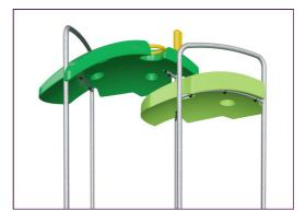
The ELEMENTS roofs are made of recyclable PE made from 33% post consumer recycled materials with a minimum wall thickness of 5 mm to ensure high durability in all climates around the world. The steel pipes are hot dip galvanised inside and outside for maximum durability.
