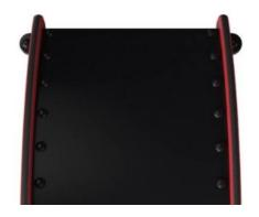
Membranes consist of friction-proof rubberized material of conveyor belt quality with excellent UV resistance. Embedded is a four-layered armouring made of woven polyester. The armouring and the two surface layers result in a total thickness of 9 mm.
