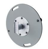
The bearing house is made from hot dip galvanised steel. The bearing shaft is made from stainless steel AISI304. The bearing itself is made from Polyoxymethylene (POM), an engineering thermoplastic with a high stiffness, low friction, and excellent dimensional stability.
