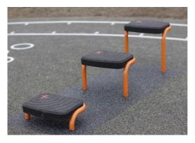
The support frame is ø48.3 x 4mm, carbon steel, with a hot-dip galvanised surface according to ISO1461, and a powder coating corrosion class C3 according to ISO12944-2. Lead content for surfaces is below 90ppm.
