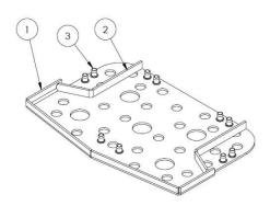
A 5 mm hot-dip galvanised carbon steel plate must is moulded inside the SBR to offer optimal stability and optimise the mounting of the step to the frame.
