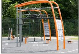
For ensuring the integrity of the main frame, the orange colored main posts are made of ø101.6 x 3mm steel posts, which are hot dip galvanized and powder coated Orange (RAL2010). The supportive posts receive the same surface treatment and are made of ø76.1 x 3.6mm steel tubes, powder coated grey (RAL7012).
