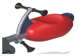
Handles and footrests are made with a moulded PP insert and an outer layer of soft TPV rubber. The handles and footrests are attached to the pipe with a galvanised steel inlay to ensure strength and durability.
