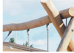
The swing hangers are made of high-quality UV-stabilised nylon (PA6) housing with integrated lifetime sealed ball bearings. The adjustable height chains are fixed by a stainless steel hook with theft-proof snake-eye bolt in a turnable anti-twist housing.
