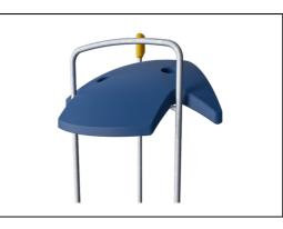
The ELEMENTS roofs are made of recyclable PE made from 33% post consumer recycled materials with a minimum wall thickness of 5 mm to ensure high durability in all climates around the world. The steel pipes are hot dip galvanised inside and outside for maximum durability.
