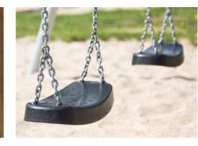
The standard seats of KOMPAN swings are engineered for maximum safety and durability. The seat two component seat with a PP inner core and outside rubber is produced in one operation. The seats are available with swing chains of either hot-dip galvanised steel or stainless steel for all swings heights.
