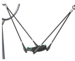
GALAXY ropes have six-stranded steel wires and a steel wire core. Each strand is tightly wrapped with PES yarn, which is melted onto each individual strand. After initial friction has been removed from the surface fibres, a harder PES coating is applied to protect each strand, making the ropes highly wearable and vandalism resistant.
