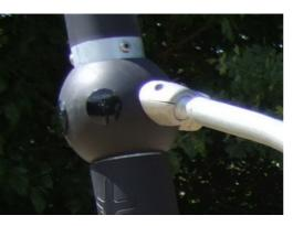
The unique designed GALAXY connection ball is produced with an inner circular core of aluminium surrounded by a shell of hard PP with an outer layer of soft TPV rubber. Flexible leadfree aluminium connectors allow for installation in variable angles.
