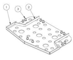
A 5 mm hot-dip galvanised carbon steel plate must is moulded inside the SBR to offer optimal stability and optimise the mounting of the step to the frame.
