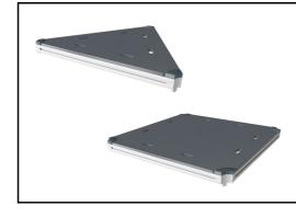
All decks are supported by unique designed low-carbon aluminum profiles with multiple attachment options. The grey colored molded decks are made of 75% post-consumer waste PP material with a non-skid pattern and texture surface.
