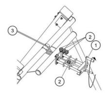
The steel cable three is tensioned by a specially designed device. By turning the handle, the steel cable can be tensioned safety. After tensioning the cable is locked by three clamps two. The tensioning device can also be used for adjustment during annual inspections.
