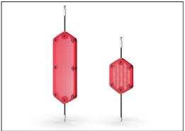
Turnable optic panels of two 7mm thick polycarbonate plates with a distance of 40mm. The inside graphic print consist of an inner image layer and outer transparent protection layer. Both PC panel and the water-based lacquer are UV stabilized to prevent fading of the print.
