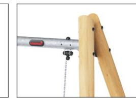
The swing hangers are made of high-quality UV-stabilised nylon (PA6) housing with integrated lifetime sealed ball bearings. The adjustable chains are fixed by a stainless steel hook with a theft-proof snake-eye bolt which is manufactured within an anti-twist house. All seats are fixed with two chains and are available with either standard or anti-wrap suspension.
