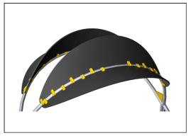
Roof is made of a steel frame supported Ekogrip® panel. The Ekogrip® panel consist of a 15mm thick PE base with 3 mm top-layer of rubber.
