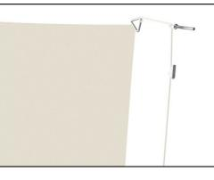
All fixation points are equipped with steel brackets to ensure strong connection to the nylon rope used for tightening.
