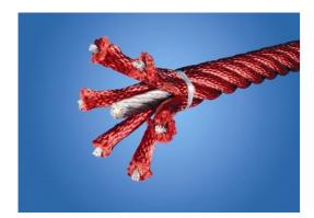
Corocord ropes with 19mm+ diameter are known as a 'Hercules' rope type which is formed from galvanised six-stranded steel wires. Each strand is tightly wrapped with PES yarn, which is melted onto each individual strand. Ropes are highly wear-and vandalism-resistant and can be easily replaced on-site if needed.
