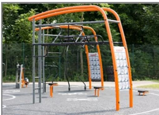
For ensuring the integrity of the main frame, the orange colored main posts are made of ø101.6 x 3mm steel posts, which are hot dip galvanized and powder coated Orange (RAL2010). The supportive posts receive the same surface treatment and are made of ø76.1 x 3.6mm steel tubes, powder coated grey (RAL7012).
