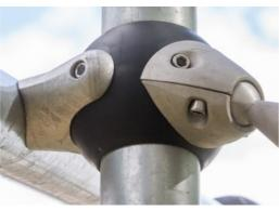
The unique designed GALAXY connection ball is produced with an inner circular core of aluminium surrounded by a shell of hard PP with an outer layer of soft TPV rubber. Flexible leadfree aluminium connectors allow for installation in variable angles.
