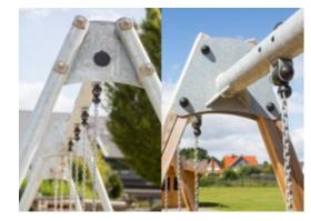
The A-Frame is designed with hot dip galvanised ø100mm crossbar with large steel end plates for strong fixation of the two post options: Hot dip galvanised ø70mm steel. Impregnated pine wood with hot dip galvanised steel footings.
