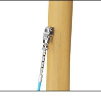
The swing hangers are made of stainless steel brackets and can move over two axis. The flange bearings are silicone enriched to make the suspension maintenance free. The connection to the rope is made with stainless steel chain.
