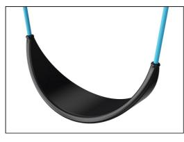
The belt seat is made of UV stabilized PUR. It retains its properties in the temperature range of -30°C to 60°C. The ropes are made of UV-stabilized PP rope with inner steel cable reinforcement and outside layer of transparent PUR.
