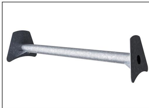
The A-Frame is designed with hot dip galvanized  $\varnothing 100$ mm crossbar with large steel end plates for strong fixation to the posts. The crossbeam is prepared for all KOMPAN hanger options.
