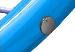
The rope is fixed to the large steel pipe by a unique KOMPAN designed tightening solution. It consists of inner and outer nylon (PA6) bushings that guides the rope to an outside threaded aluminum part that tighten the rope. Colored steel components have a base of hot dip galvanization and a powder coated top finish. This provides an ultimate corrosion resistance in all climates around the world. Other steel surfaces are hot dip galvanized inside and outside with lead free zinc.
