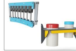
The Xylophone music panel consist of HDPE material in 19mm EcoCore<sup>™</sup> made with +95% recycled post-consumer material from e.g., food packing waste in both core and colorful outer layer. The pipes are made of die cast aluminum specifically alloyed for outdoor environments. The percussion panel consist of 2 Conga Drums with PP tubes and top in colored ABS.
