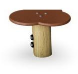
The steps are made of 21.5mm thick plywood made from alder and pine wood. Both sides are covered by 2 layers of phenolic film with anti slip net pattern. All cutting edges are sealed with paint to ensure long lifetime.
