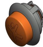
The push buttons and the housing for the push buttons are made from Polyamide (PA6). The buttons contain a magnet which activates a contactless reed switch when the buttons are pushed. This ensures high durability of the system.
