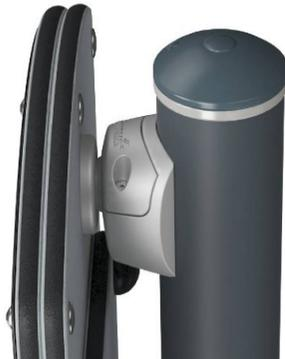
The connectors are made of die-cast aluminum specially alloyed for outdoor environments and with a lead content below 100ppm. The connectors are attached to the posts by stainless steel screws and well protected against corrosion by special designed zinc washers. Extremely strong and no change of corrosion.
