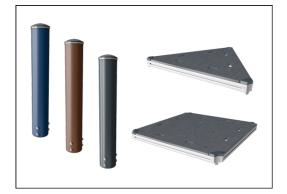
The main posts are made of high quality pregalvanized steel with powder coated top finish. Post tops are closed with caps of UV stabilized nylon (PA6). The grey colored moulded decks are made of 75% post-consumer ocean waste PP material with a non-skid pattern and textured surface. All decks are supported by uniquely designed, low-carbon aluminum profiles with multiple attachment options.
