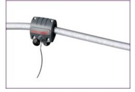
The hang-on puller is designed with at welded steel core and covered with low-density PE housing. The two rubber coated handles are angled to provide best possible ergonomic while gliding. The wheels of the puller are made of low noise TPU and installed with sealed ball bearings.
