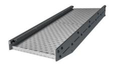
The ramp is mounted under a 15 degree angle and has a length of 2300mm. The ramp is made from 5mm aluminium plate with an anti-slip pattern.
