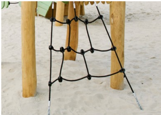
Nets and ropes are made of UV-stabilised PA with inner steel cable reinforcement. The rope is induction treated in order to create a strong connection between steel and rope which leads to good wear resistance.
