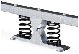
KOMPAN's springs are manufactured from highquality spring steel. The springs are cleaned by phosphating before being painted with epoxy primer and polyester powder coating. The springs are fixed by unique anti-pinch fittings for maximum safety and longevity.
