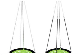
The seat suspensions are available in stainless steel chain or rope options. The ropes are made of UV-stabilised PA with inner steel cable reinforcement. The rope is induction treated to create a durable connection between the steel and rope, resulting is longevity.
