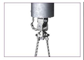
The 360-degree rotating swing hanger is made from stainless steel, and all moving parts are lifetime sealed and lubricated. The hanger system is equipped with a safety chain to prevent the swing hanger from falling if damaged.
