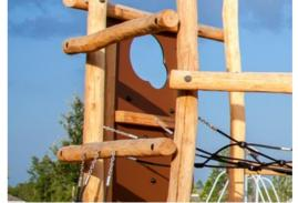
Plywood climbing panel. The climbing panels is made of 21,5mm thick plywood made from alder and pine wood. Both sides are covered by 2 layers of phenolic film with anti slip net pattern. All cutting edges are sealed with paint to ensure long lifetime
