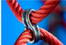
Designed to allow the typical function of rope play structures to move Corocord 'S' clamps are used as universal connections in Corocord products. 8mm stainless steel rods with rounded edges are pressed around the ropes with a special hydraulic press, making them the ideal connector. Our clamps are safe, durable and vandalism-proof.
