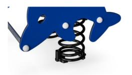
KOMPAN Springs are made of high quality spring steel according to EN10270. The springs are cleaned by phosphating before they are painted with an epoxy primer and a polyester powder coating as top finish. The springs are fixed by unique anti pinch fittings for maximum safety and long lifetime.
