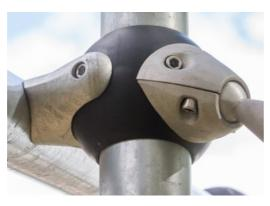
The unique designed GALAXY connection ball is made with an inner circular core of aluminium surrounded by a shell of hard PP with a outer layer of soft TPV rubber. Flexible lead free aluminium connectors allow for installation in variable angles.
