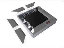
As a unique feature the SBR tiles can be removed for cleaning and service. By loosen six screws the SBR tile can be lifted up to open and gain access to the springs (see instruction on KOMPAN Master).
