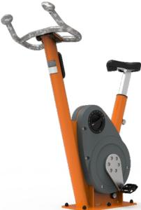
The front tube for the frame is made of S235 hot-dip galvanized steel tubing with the following dimensions Ø76,1x3,6mm. and with a powder coating corrosion class C3 according to ISO12944-2.
