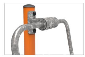
The resistance is controlled by heavy duty scaled ROSTA torsion spring element. The ROSTA element works without any noise and are maintenance free. The ROSTA element allows the user to both push and pull depending on the desired exercise.
