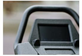
The handle bars are designed with multiple hand positions to accommodate different postures and riding styles. It is a casted aluminium part with polyurea coating for good grip and insulation.
