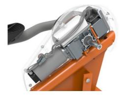
The innovative self-powered electrical motor and gear provides a virtual flywheel to give real road cycle experience. The resistance works as an automatic drive and adapts automatically. The users can overwrite the automatic drive manually by changing the resistance in 10 steps (45-750 Watts) through KOMPAN's fitness app or on screen.
