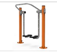
The arms for the foot pedals are 855mm long, and made from ø48,3x4mm S235JR hot dip galvanized steel tube.
