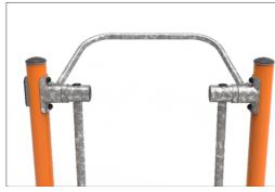
Safety bar is made of tubing with a diameter of 38 mm and wall thickness of 2 mm made of steel S235 with a hot dip galvanized surface treatment according to ISO1461 with a lead content below 90ppm for surfaces and for base material below 100ppm and with powder coated top finish.
