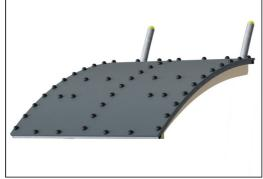
Roof is made of a steel frame supported Ekogrip® panel. The Ekogrip® panel consist of a 15mm thick PE base with 3 mm top-layer of rubber.
