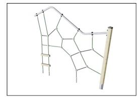
Corocord ropes of UV-stabilized PES rope strands with inner steel cable reinforcement. The polyester yarn is made from +95% post-consumer materials and is inductively melted onto each strand. PES has high strength with excellent resistance to abrasion and UV radiation. The rope loops are assembled by aluminum connectors.
