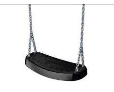
The standard seats of KOMPAN swings is engineered for maximum safety and durability. The two component seat with a PP inner core and outside rubber is produced in one operation. The seats are available with swing chains of either hot dip galvanised steel or stainless steel for all swings heights.
