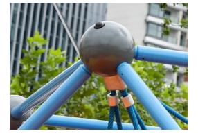
The metal parts are made of high quality steel, hot dip galvanised inside and outside with leadfree zinc. On the outside, there is an additional layer of powder coating. This ensures both excellent corrosion resistance and colourful design expression. LUNA
