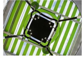
Corocord membranes consist of friction-proof rubberized material of conveyor belt quality with excellent UV resistance. Tested and compliant with REACH requirements for PAH. Embedded is a four-layered armoring made of woven polyester. The armoring and the two surface layers result in a total thickness of 7.5 mm.
